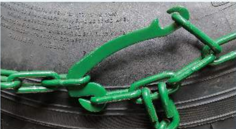
Locking lever system,the key component used to tighten the snow chain firmly
